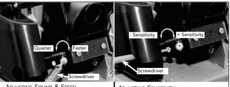
ADJUSTING SOUND & SPEED The dryer is shipped set at maximum speed. Turn counterclockwise to reduce sound and speed. 3/4 of a turn max.
